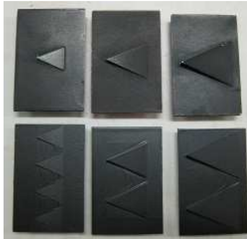
Figure 3.14: Photo of all six models, single configuration (top) and array configuration (bottom) painted with black-matte paint.
