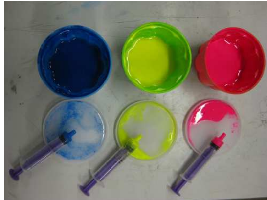
Figure 3.27: Three different fluorescent colours prepared for oil-flow visualisation.
