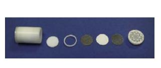
Figure 8: An Ogawa personal air sampler <sup>51</sup>
