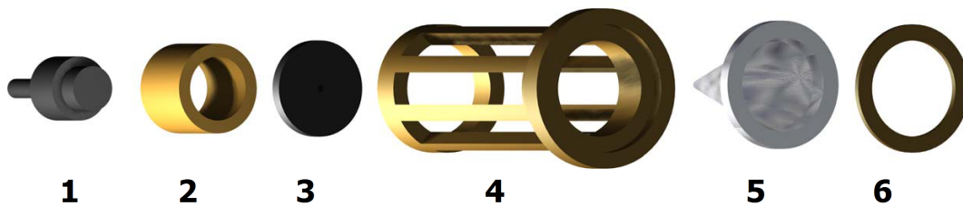
Figure 3.7: The molecular beam apparatus. 1 - Molecular beam valve. 2 - Brass tube. 3 - Molecular beam nozzle. 4 - “Birdcage.” 5 - Skimmer. 6 - Brass cap.
