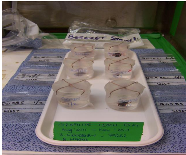
Figure 18: Leaching experiment set -up
