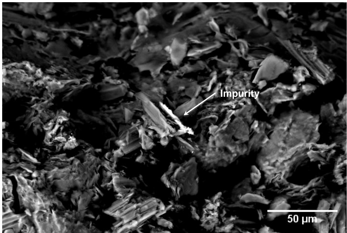
Figure 47: Back scattered electrons (BSE) micrograph of PGA graphite showing a selected impurity – Scale bar 50 \mu\text{m}
