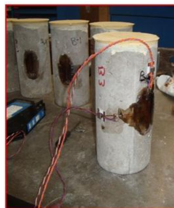
Figure 3.7: Layout of instrumentation of FRP tubes confined concrete and unconfined cylinders
