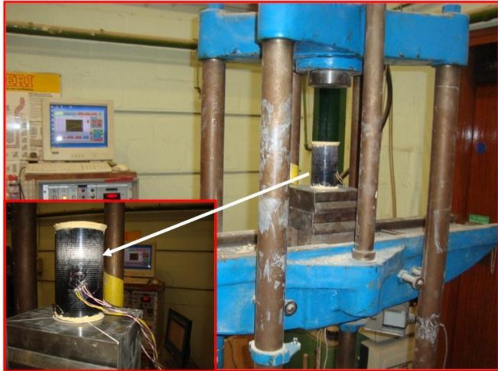
Figure 3.8: FRP-Tube Confined Concrete testing set-up
