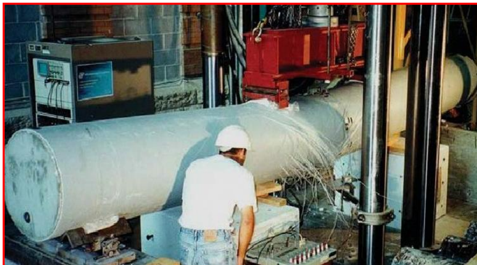
Figure 2.17: Tests set up for bending tests on FR pile (Fam and Rizkalla, 2003)
