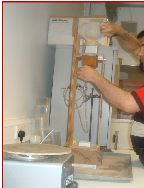
Figure 4.5: Schematic view of the: a) Sand Raining Frame. b) Sand preparation
