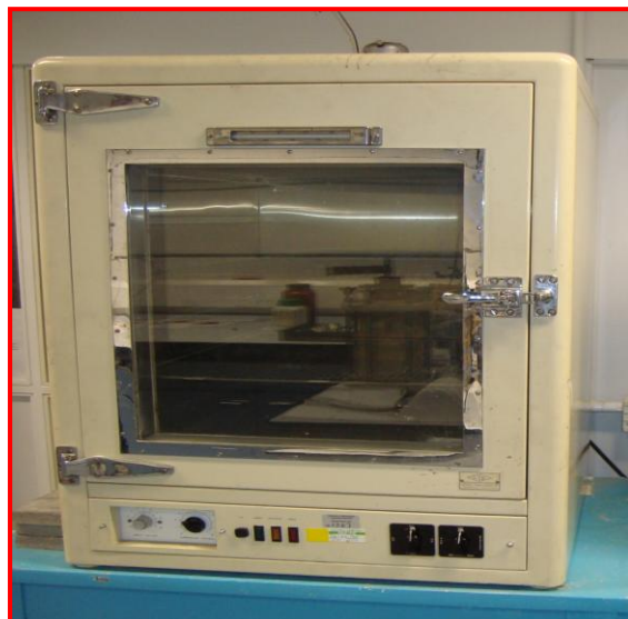
Figure 3.26: Oven used for acceleration process
