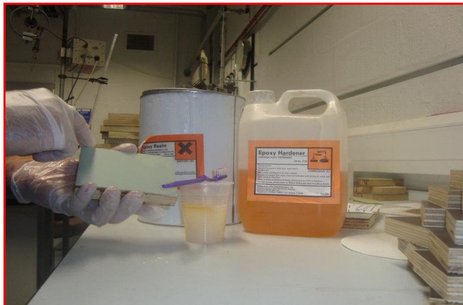
Figure 4.17: GFRP plate glued to the timber block
