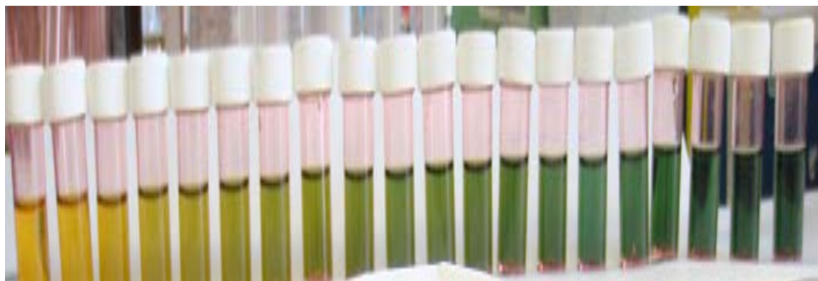
Figure A2.1. Colour change observed with increasing concentrations of PVA from yellow to green in a colorimetric assay of PVA (0 to 0.1 mg ml -1 ).
