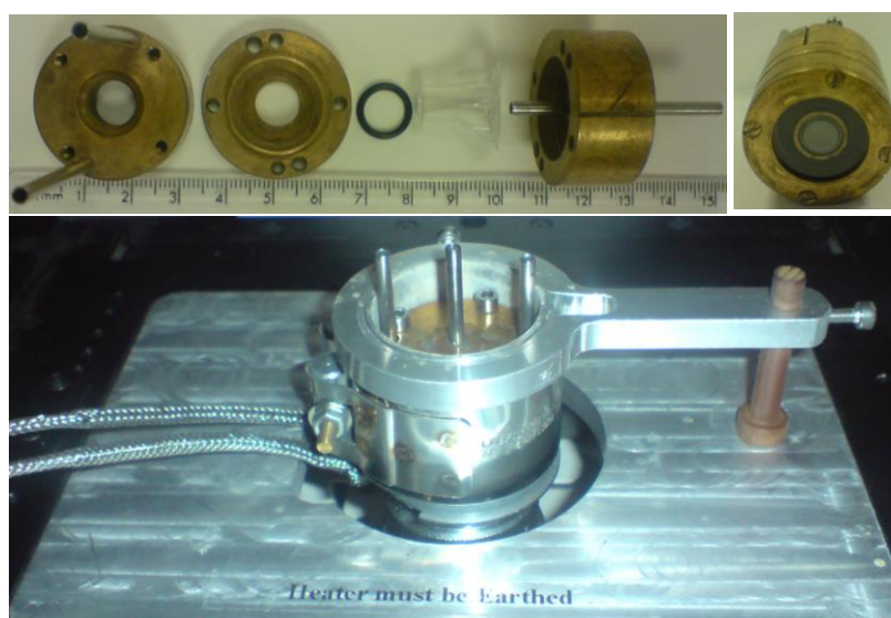
Figure 4.1 The flow cell chamber and heating stage setup utilised in the real time characterisation of BSA-AF488 monomer loss following heating at 50 ^{\circ}\text{C} . 21
