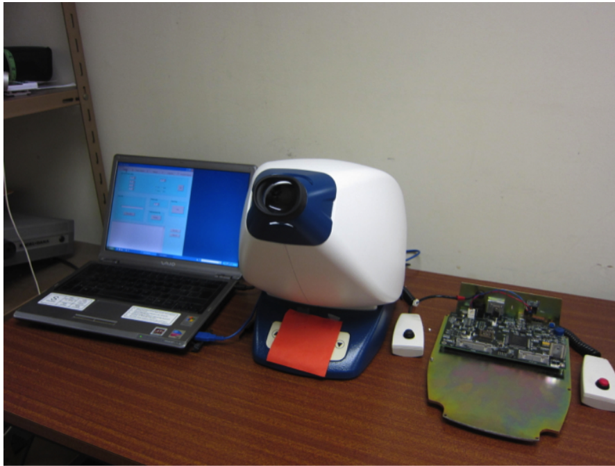
Figure 7.2.1: The device is seen in the centre of the image and the laptop that drives the controlling software is on the left. The white subject response button is to the right of the device. The main board with control electronics is on the right. Its (red) response button is at the far right.
