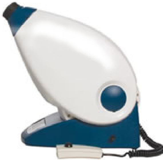
Figure 2.6.1: The digital dark adaptometer, a modified MPS9000 (Hartest Precision Instruments, Crawley, UK)
