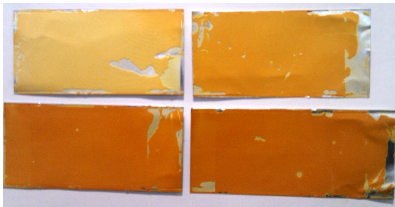
Figure 3.29: Mechanical damage to several initial TLC plates after 10 runs of the shock tube
