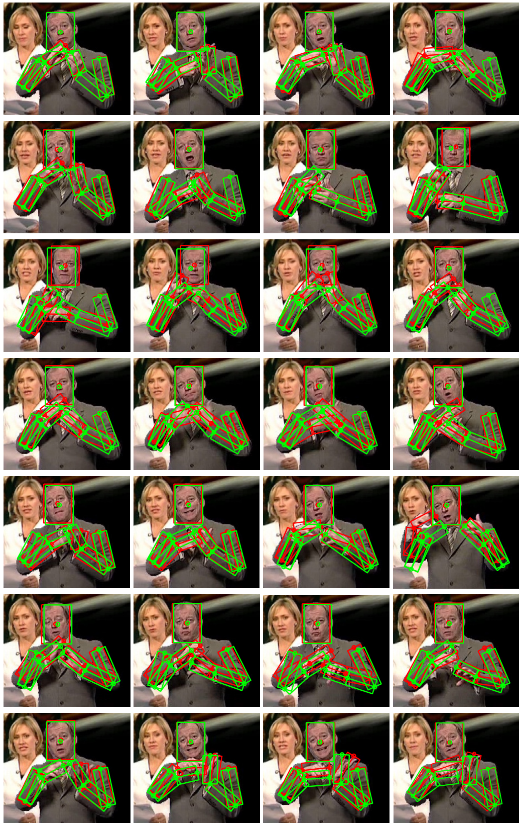
Figure 4.7: Tracking results for the sign language dataset showing every fifth frame of a continuous sequence. Ground truth shown in red, predicted pose is shown in green.
