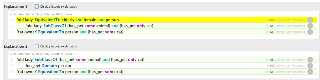
Figure 2.12: Two example justifications for the entailment 'old\ lady' \sqsubseteq 'cat\ owner' as they are presented in Protégé 4.
