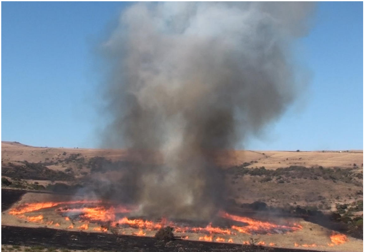
Figure 7.1: Plume generated by a spiral ignition in a 4 ha plot in South Africa in June 2012.
