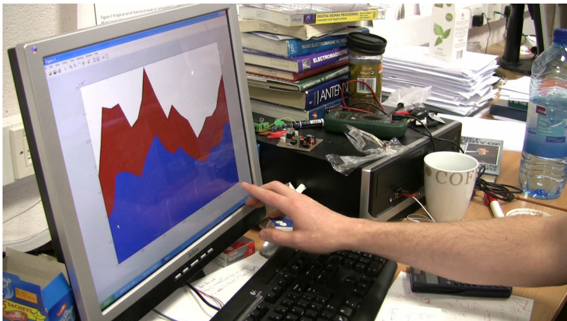
Figure 11 – A 'stacked' graph, comparing data taken of a non-metal object (blue) with the same non-metal object plus an added metal component (red)
