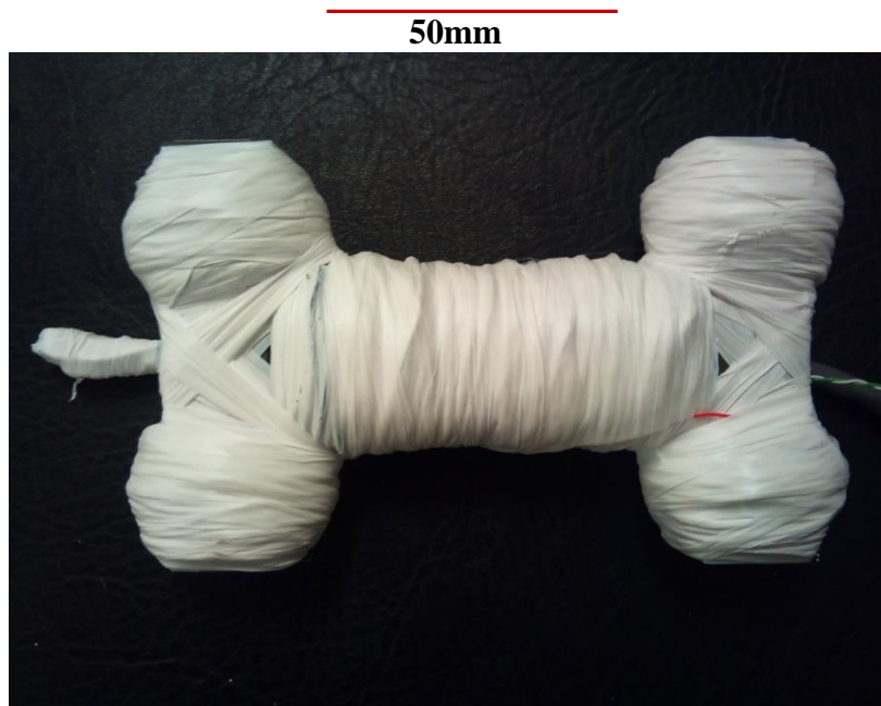
Figure 7.13 Re-wound Sensor Head for the 200 Hz to 24 kHz frequency range.
