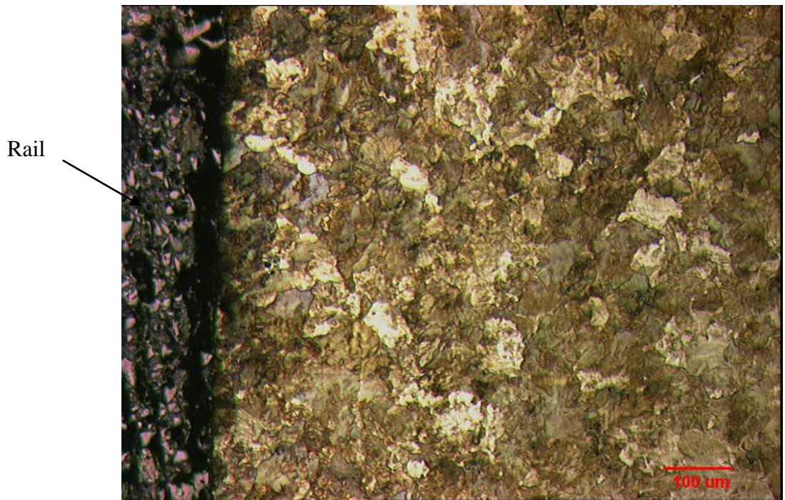
Figure 0.7 Optical Micrograph showing (a) 610 µm decarburisation layer (b) minimum decarburisation layer (none)
