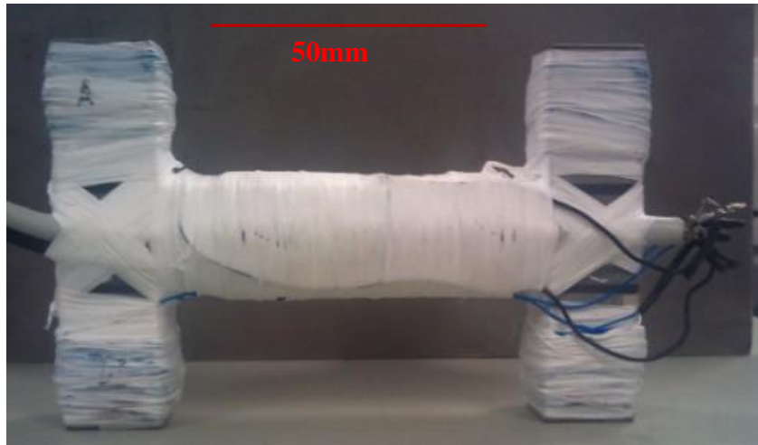
Figure 7.3 Sensor head working between 800 Hz to 100 kHz
