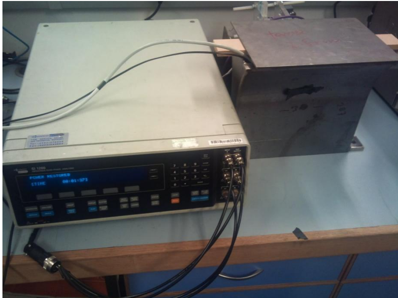
Figure 7.27 Measurement setup including the impedance analyser and the metallic housing
