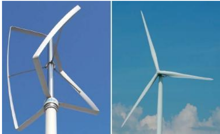
Figure 2-6 Lift-driven wind turbines: VAWT and HAWT (Example)
