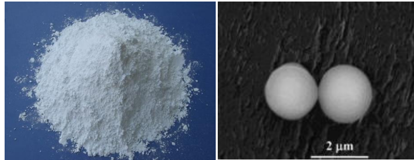
Figure 3.2 Fused silica particle used in this study (a) powder (b) SEM picture for the particle with 1.5 \mu\text{m} diameter manufacturer,supplier
