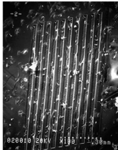
Figure 2.13 The surface of stent after micro fabrication for anti-growth of protein [135]
