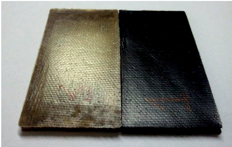
Figure 7.10: Example of a Moulded Piece Produced from Uncoated and RFL Coated Fabric using an Open Flash Mould
