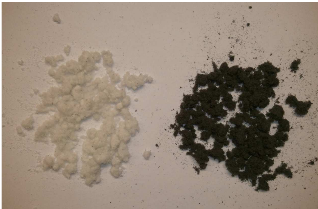
Figure 8.5: Uncoated (left) and Coated (right) Beaten Waste Fabric used in Rubber Processing
