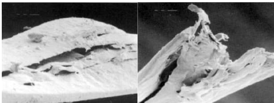
Figure 4.39: SEM Micrograph of Nylon Fibres Broken due to Impact (Hearle, 1998).
