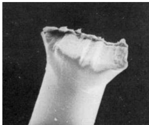
Figure 4.38: SEM Micrograph of Polyester Cut with Scissors (Hearle, 1998)
