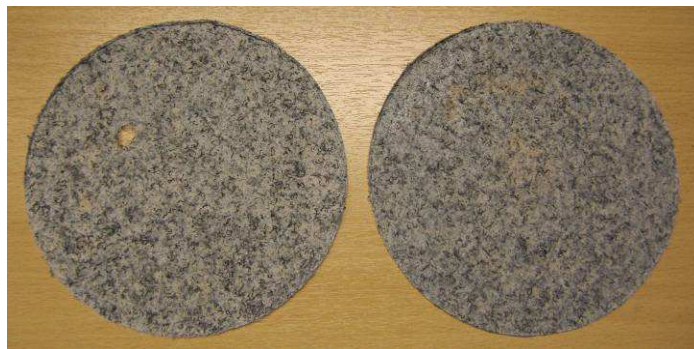
Figure 5.12: Photographic examples of sheets with minor faults such as the hole in the left sheet and small areas of thinness in the right sheet.
