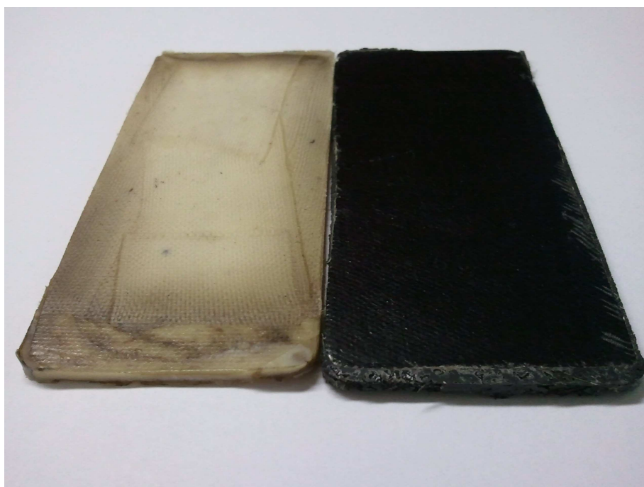
Figure 7.11: Example of a Moulded Piece Produced from Uncoated and RFL Coated Fabric using a Positive Mould
