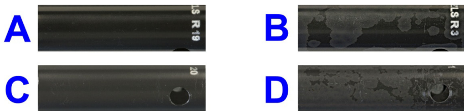
Figure 7: Autoclave corrosion weight gain profile of non-hydrided ZIRLO™ SR and RX materials. Photographs of actual corrosion specimens included: (A) non-hydrided ZIRLO™ – SR after 60 days of autoclave exposure, (B) non-hydrided ZIRLO™ – SR after 140 days, (C) non-hydrided ZIRLO™ – RX after 80 days and (D) non-hydrided ZIRLO™ – RX after 160 days.
