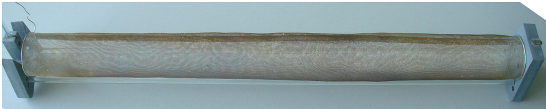
Figure 2: Basket shaped Pt counter electro used during hydrogen charging.
