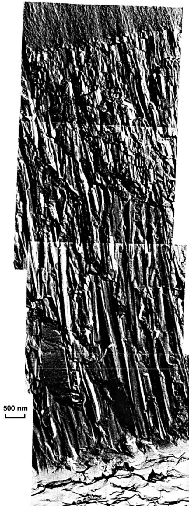
Figure 2: Columnar oxide crystallite growth on Zr after 24hr in 600°C air [48]. Oxide-metal interface is at bottom. Micrograph is from a two stage (Formvar/carbon) replica of the oxide fractured (after dissolution of the Zr matrix) by gluing the oxide to a glass microscope slide, scribing the back surface of the slide, and fracturing the composite of slide and oxide.
