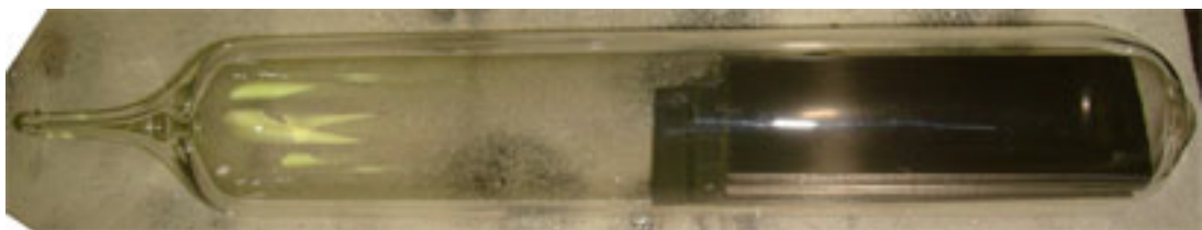
Figure 30: Sheet ZIRLO™ samples in a quartz capsule awaiting stress relieve anneal.
