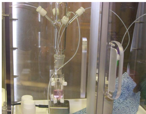
Figure 2.4: ^{243}\text{Am}^{\text{III}} sample preparation in custom made test tube. The right hand side tube pumped the sample out of the test tube, and the left hand side tube pumped the sample back into the test tube.
