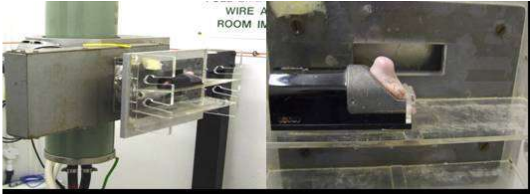
Fig. 2.1 Tumour irradiation apparatus. The image on the left shows a side-view of the MXR-320/36 X-ray apparatus with a tumour bearing mouse (X-rays were delivered in the horizontal plane). The image on the right shows a tumour bearing nude mouse in a polyvinyl restraining jig (black) with lead shielding (grey) with maximal exposure of the tumour to the X-rays and minimal exposure to other tissues.
