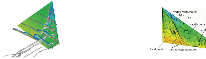
Figure 9. Visualisation of instantaneous vorticity (left) and time averaged streamlines (right) of the Implicit LES simulation of Hahn & Drikakis (2009).
