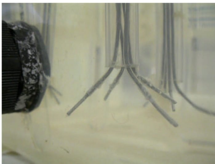
Figure 3-35: Thin calcareous deposit on sample polarized at -950 mV
