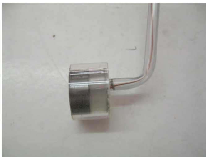
Figure 3-1: Front view of the mounted coupon
