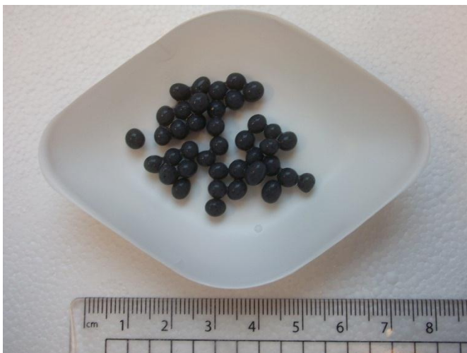
Figure 3.4: Alginate beads containing immobilised palladised E. coli .
