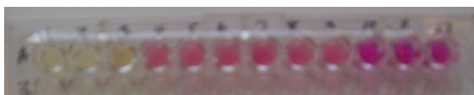
Figure A2.2: Colorimetric plate assay, demonstrating the complete reduction of the pyrogallol red dye by horseradish peroxidase (wells 1-3), with partial reduction in wells 4-6 (no MTQ substrate) and wells 7-9 (no biocatalyst), and no reduction in wells 10-12 (no HRP).
