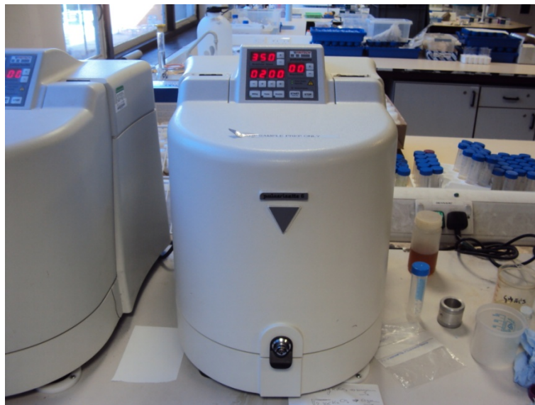
Figure 3-1 Pulverisette 6 planetary mill used for mixing.
