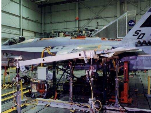
Figure 1.23: Active Aeroelastic Wing subject to torsion tests [146].
