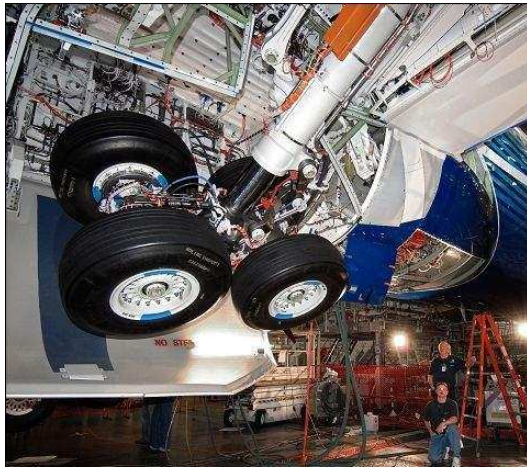
Figure 1.12: Retractable undercarriage of a Boeing 787 [145].
