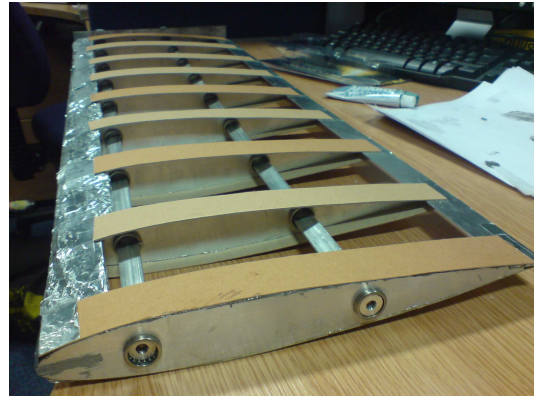
Figure 5.11: Leading-edge profile and rib caps.
