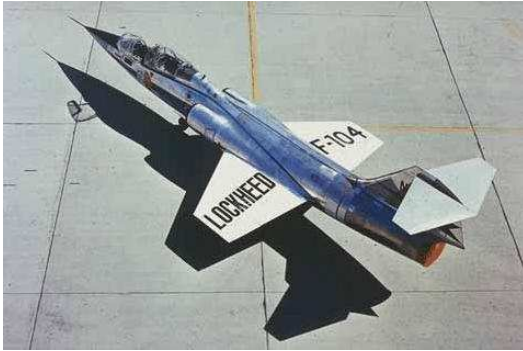
Figure 1.3: The small wing area and aspect ratio of the Lockheed F-104 [170].
