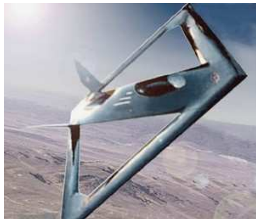
Figure 6.2: A joined-wing HALE UAV concept [152].
