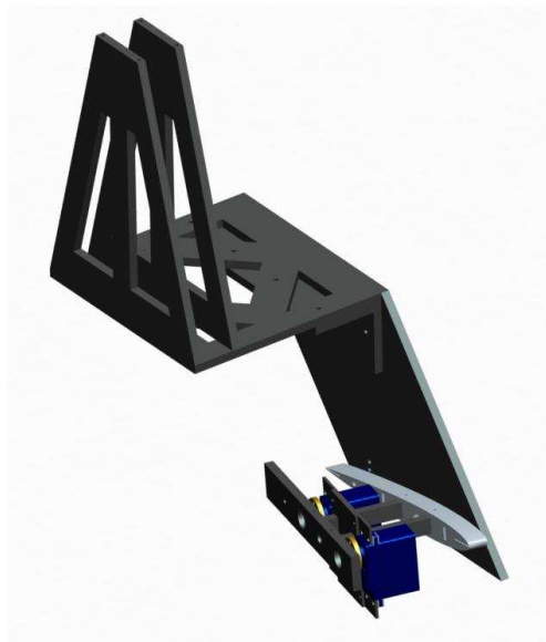
(a) CAD model of the wing mount with actuator housing and servos attached.
