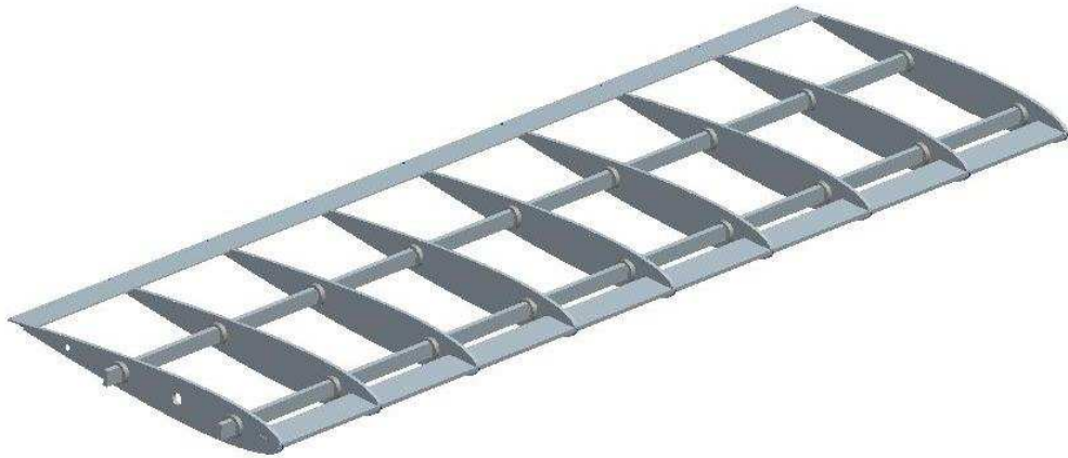
Figure 5.1: CAD model of the wing design.
