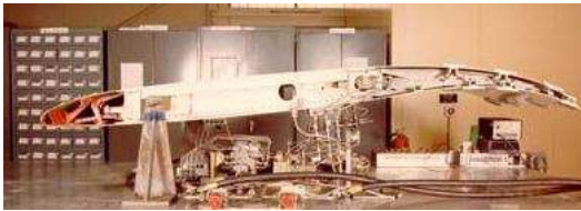
Figure 1.19: The internal structure and actuators of the compliant Mission Adaptive Wing for enabling variable camber with surface continuity [137].
