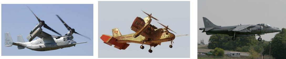
(a) Bell-Boeing V-22 tiltrotor [148]. (b) Canadair CL-84 tilt wing [154]. (c) Hawker Siddeley Harrier GR7 vectored thrust [153].
