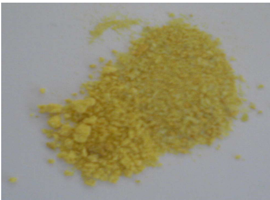
Figure 7.2 Product obtained after decomposition of fully cured samples of Araldite DLS 772 / 4 4' DDS with an amine / epoxy ratio of 0.8 after decomposition at 120 °C for a total of 75 minutes in Microwave Reaction System.
