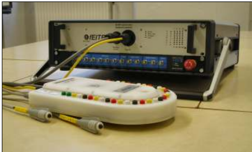
Figure 2.5 A photograph of the fEITER system, including the Base Unit with the stimulus generator, the HeadBox and the independent switches (emergency stop and user input mode control).
