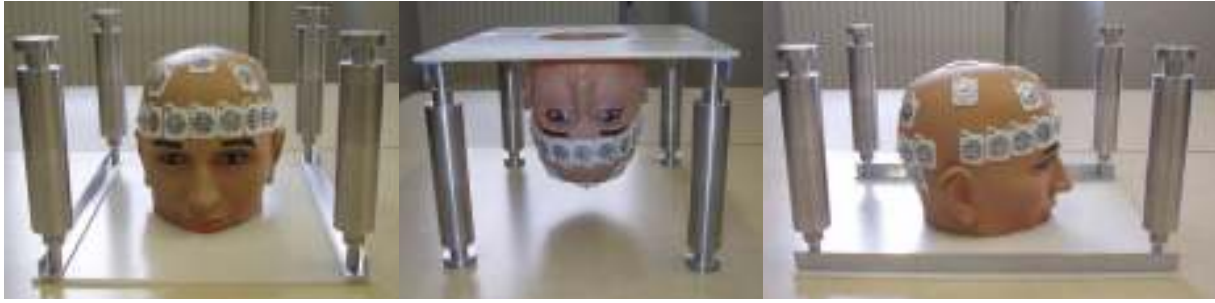
Figure 5.1 Photographs of the head phantom used for fEITER tank tests.
