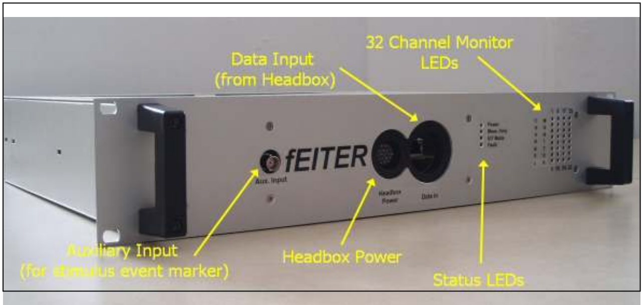
Figure 21.1.11 Photograph of the external view of the inner base unit casing, showing the 32 LED monitor channels, the data input and headbox power sources.
