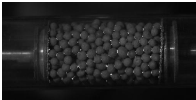
Figure 2.8: Image of plasma generation in a packed-bed DBD reactor, showing microdischarges at the contact points between \text{BaTiO}_3 beads.
