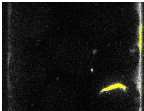
Figure 3.26: Microscope-ICCD images of a) BaTiO 3 beads, b) spots of plasma generation at contact points between BaTiO 3 beads and c) streamer extending over the surface of a BaTiO 3 bead.
