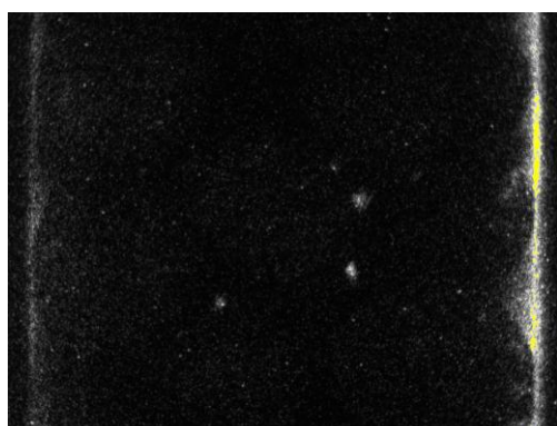
Figure 3.26: Microscope-ICCD images of a) BaTiO 3 beads, b) spots of plasma generation at contact points between BaTiO 3 beads and c) streamer extending over the surface of a BaTiO 3 bead.
