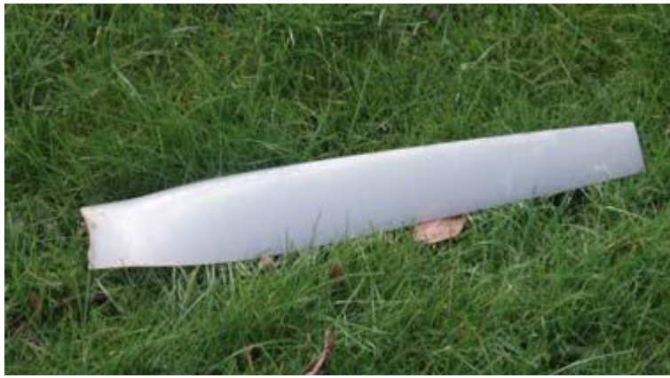
Figure 12.13: Damaged turbine blade which had detached during the storm on 18 th January 2007
