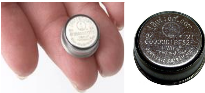
Figure 6.5: IButton temperature/humidity recorder
