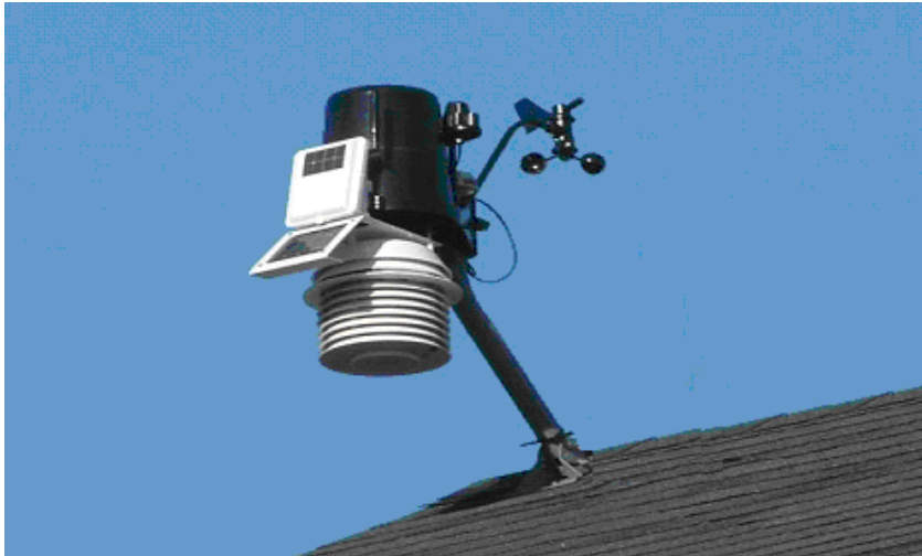
Figure 6.1: Davis Vantage Pro 2 Plus Weather Station at EcoSmart village
