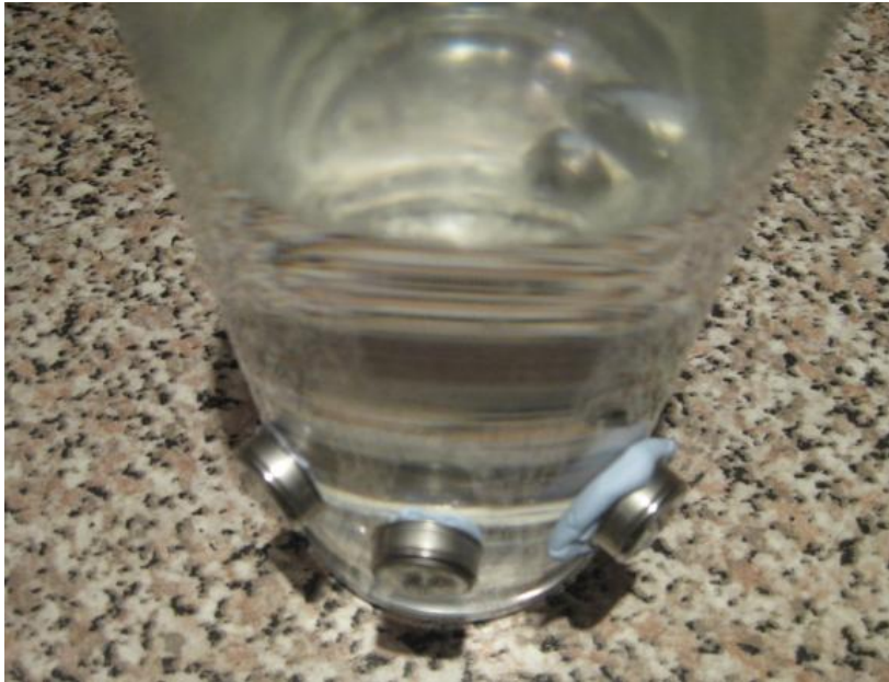
Figure 6.7: Testing thermal effects of using Blu-Tack to attach IButtons
