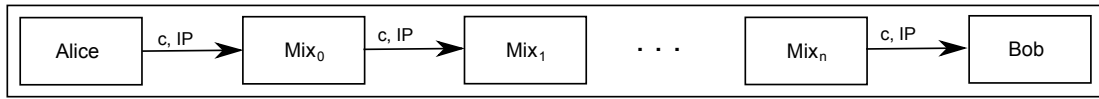
Figure 3.1: A simple mix system used by Alice to send ciphertext c to Bob. c is the encryption of a message using Bob's public key.
