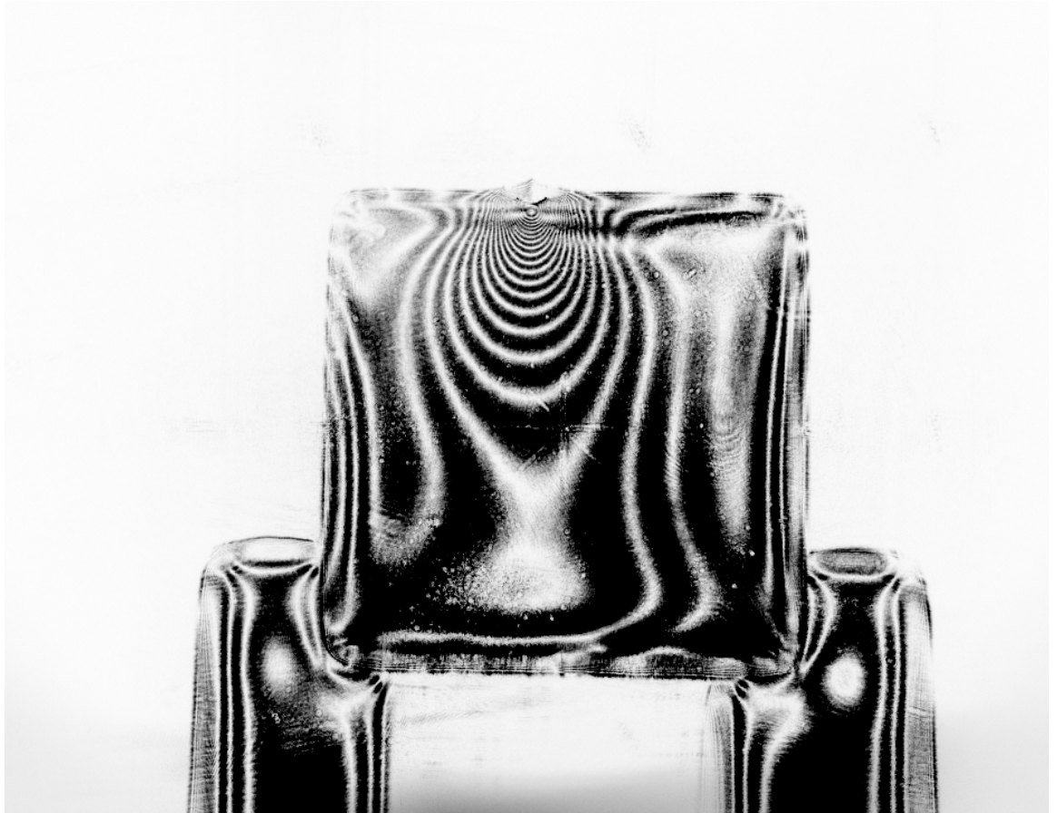
Figure 3.1: Epoxy resin cube with a point load, viewed through a polarizing filter [Image courtesy of Rachel Tomlinson, University of Sheffield]
