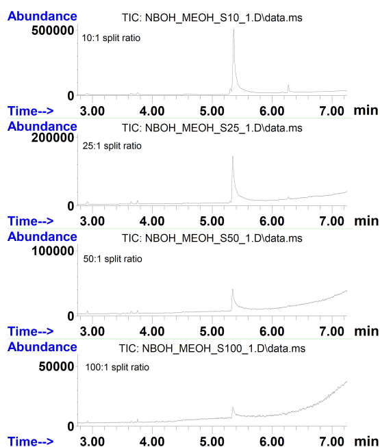
Fig. 3: TICs obtained from a methanol extract of one single blotter paper using different injection split ratios
