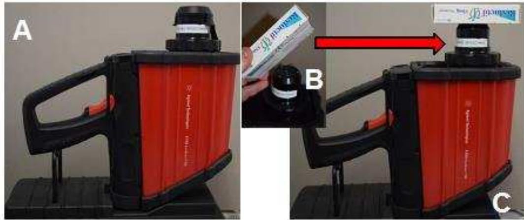
Figures 2.6a to c - Docked ExoScan Analyser for Lap Top Communication with a Specular Reflectance Measuring Head in a) Referencing Mode, b) Sample Placement, and c) Suspect Analysis Mode post
