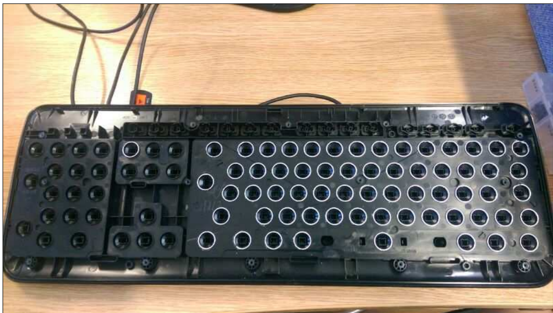
FIGURE 6.1: The disassembled keyboard with white paint highlighted keys
