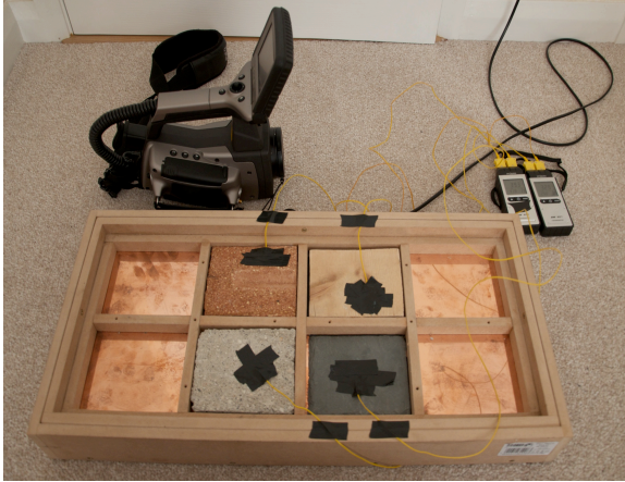
Figure 2 Photo of the experimental setup, thermocouples and IR camera
