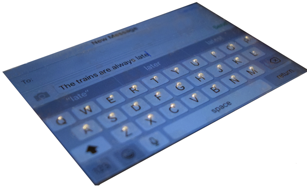
Figure 3. Tactile overlay consisting of a semi-rigid screen protector modified with braille-like bumps to provide passive tactile feedback regarding key position.
