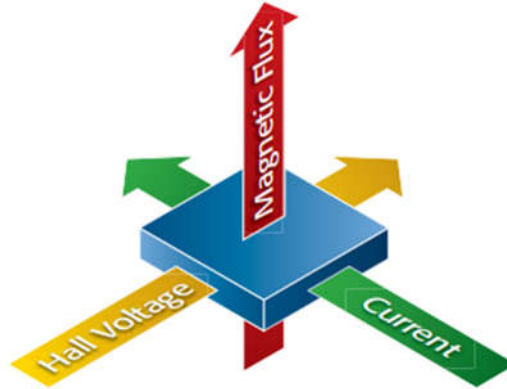
Figure 6. Illustration of Hall Effect [15].
