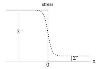
**Figure 4.** Schematics illustrating the spatial distribution of initial stress utilized in obtaining the analytical solution of Equations (6) (solid line) and the numerical solution of Equations (7) (dotted line).
