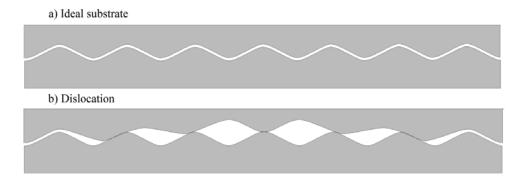
**Figure 3.** Schematic illustration of the dilatancy effect due to the presence of a macroscopic dislocation: (a) frictional surfaces in contact in the case of an ideal substrate (seven sinusoids at the top and bottom surfaces); (b) the same substrate with single dislocation (seven sinusoids at the bottom surface and six at the top surface).
