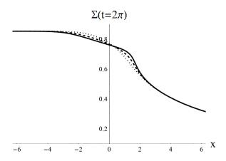
**Figure 10.** Spatial distribution of shear stress at  $t = 2\pi$  for various values of the dissipation coefficient C defining a velocity-dependent friction  $f = Cu_t$ : C=0.1 (solid line), C=0.5 (dashed line) and C=2.0 (dotted line). The initial stresses are  $\Sigma^-=0.855$  and  $\Sigma^+=0.179$ .
