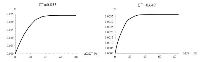
**Figure 13.** Slip velocity at position x = 0 as a function of  $\Delta \Sigma / \Sigma^-$  for two values of initial shear stress  $\Sigma^-$ .
