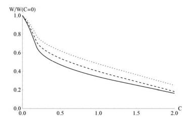
**Figure 11.** The ratio of slip velocity  $W(C \ge 0)$  to slip velocity with no dissipation W(C = 0) as function of dissipative coefficient C for various values of shear stress,  $\Sigma^- = 0.855$  (solid curve),  $\Sigma^- = 0.606$  (dashed curve) and  $\Sigma^- = 0.419$  (dotted curve). Increasing friction significantly decreases the slip velocity, with a weak dependence on the initial shear stress  $\Sigma^-$ .
