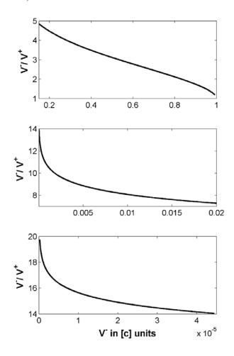
**Figure 5.** Ratio of fast rupture velocity  $V^-$  to slow rupture velocity  $V^+$  as a function of  $V^-$ . Both fast and slow velocities decrease with decreasing shear stress, but the latter velocity decreases more quickly. Thus, for processes such as slow slip events the slip pulse increases in extent essentially from one side.
