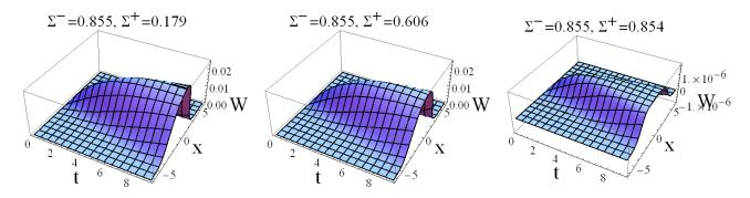
**Figure 12.** Spatial and temporal distribution of slip pulse velocity for various values of the coefficient  $\Sigma^+$  (dissipation coefficient 0.1).
