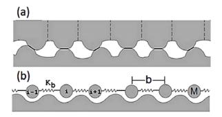
**Figure 1.** Schematic of asperity contact (a) and chain of masses interacting via elastic springs and placed in a periodic potential (substrate) (b). The balls represent asperities. The sine-shaped surface is the opposite plate.
