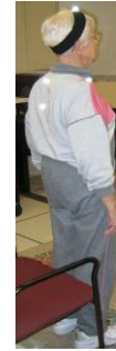
Fig. 7. An elderly participant with markers on the head, shoulder, two on the back and feet for the VICON motion capture system.
