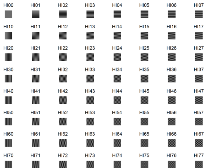
FIGURE 6 – DCT 8X8 BASIS IMAGES
