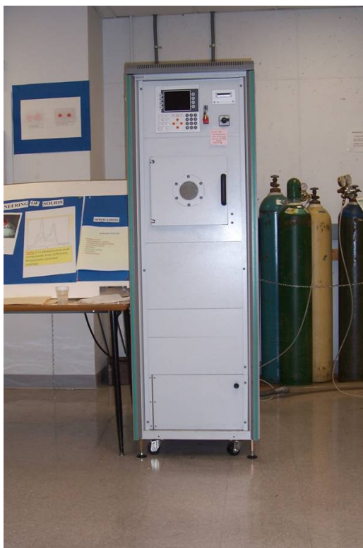
Figure 2.1: Plasma Tech coating microwave used for HMDSO plasma coating.
