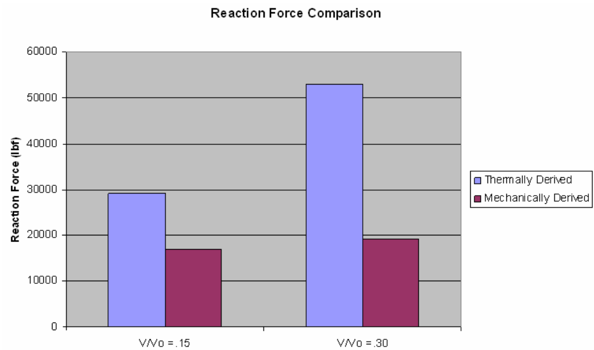
Figure 4.19. Reaction force comparisons for thermally and mechanically derived stiffeners for two volume ratios.
