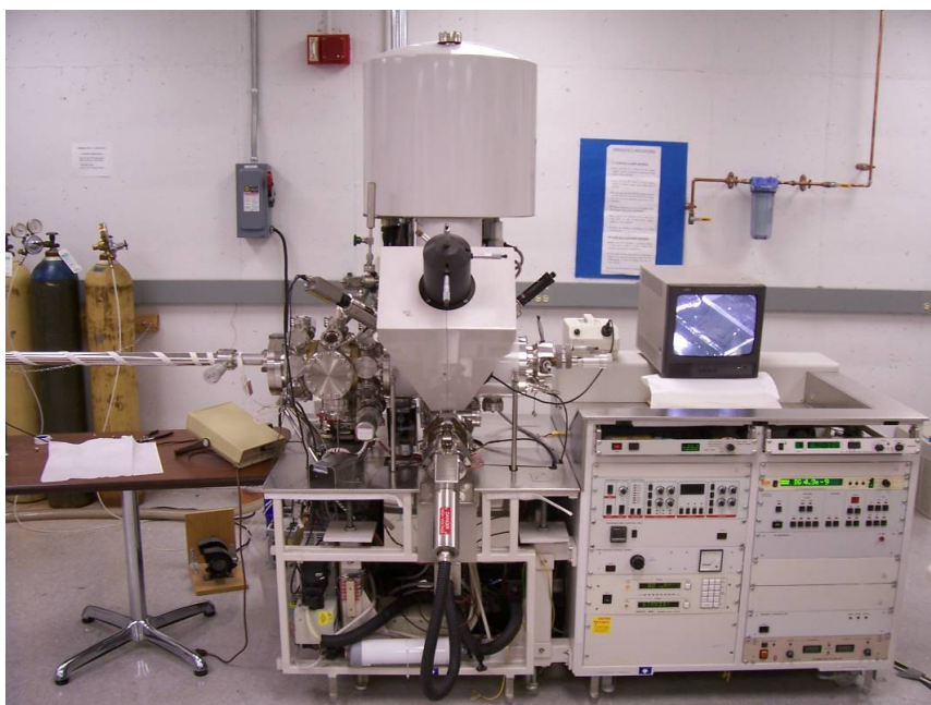
Figure 2.11: XPS AXIS ULTRA from KRATOS ANALYTICAL Inc. (funded by NSF and OBR)
