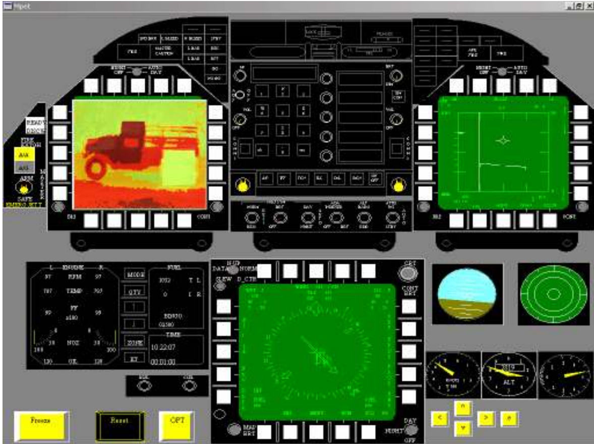
Figure 15: Combat simulation instrument panel. Images are displayed on the top left, waypoint headings in the bottom center, and threats on the center left.
