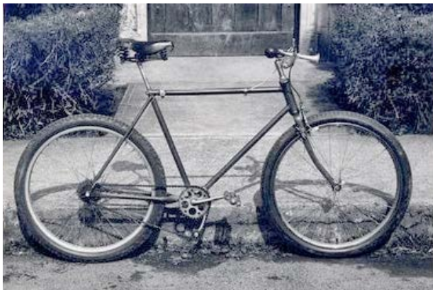
Figure 1. John Finely Scott's "Woodsie" assembled in 1953 using a Schwinn World diamond frame, balloon tires, flat handlebars, and derailleur gears. Reproduced with permission from Marin Museum of Bicycling.
