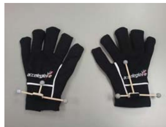
Data gloves used as input devices with attached marker spheres for optical tracking
