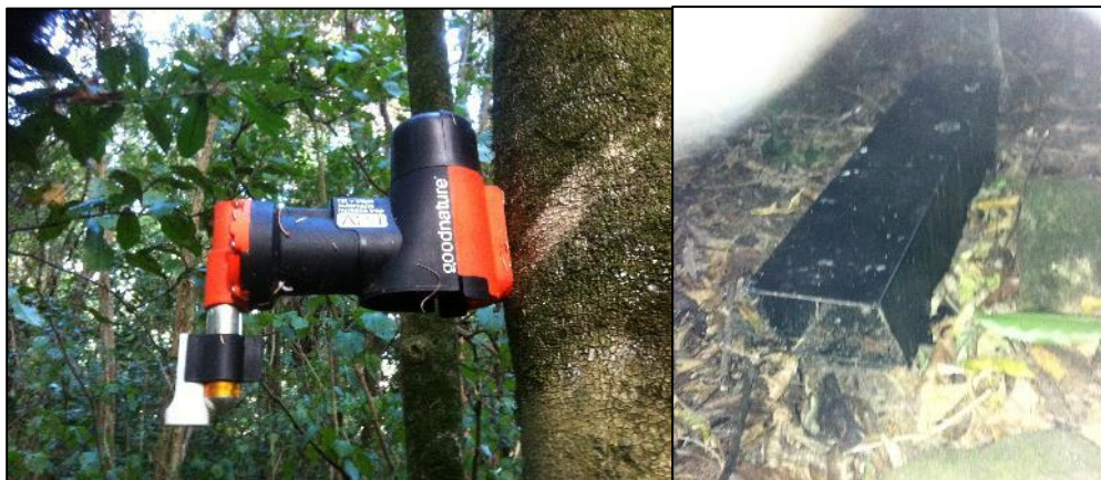
Figure 7.20 Left: The A24 rat and stoat trap by Goodnature (n.d.). Right: A tracking tunnel, seemingly not in use (no lure or paper inside). Both were likely installed by the Little River Trap library.
