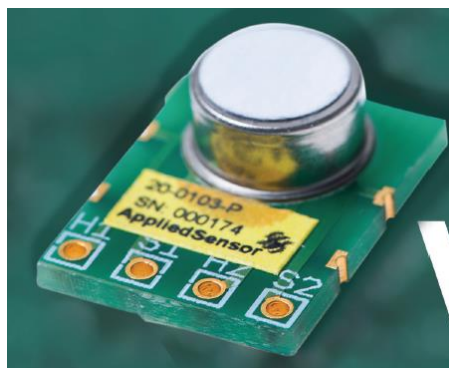
Figure 6.6: Appliedsensor AS-MLV-P sensor body (13)
