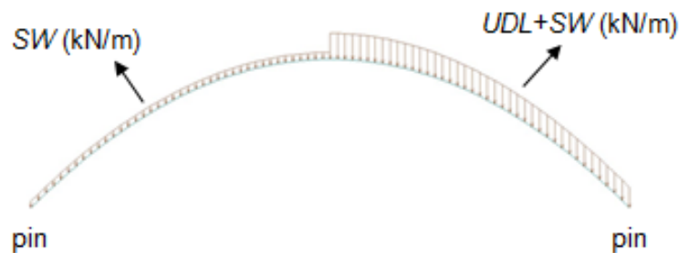
Figure 3.4. FE : The load pattern of 20 kN/m UDL applied across the half span of the arch plus SW
