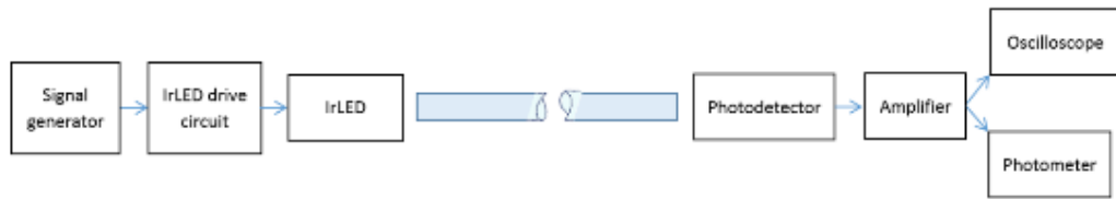
Figure 4-5 Channel measurement experimental setup
