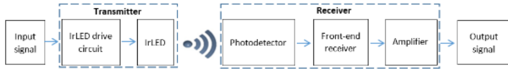
Figure 3-1 OW communication system
